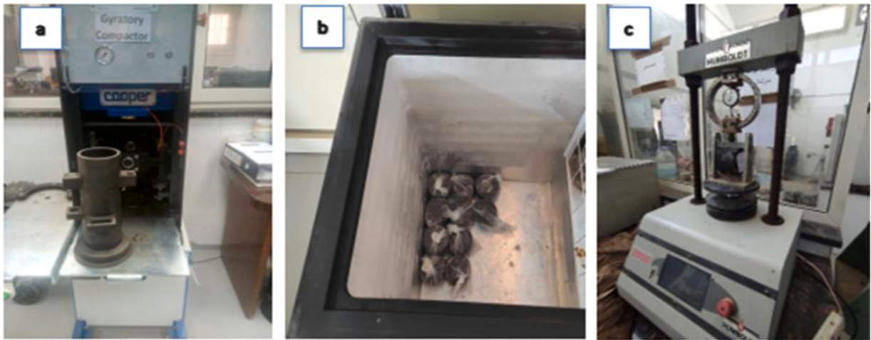
Fig. 7. The device was used in ITS test, (a) gyratory compactor; (b) sample in freezer; (c) sample in ITS machine.
